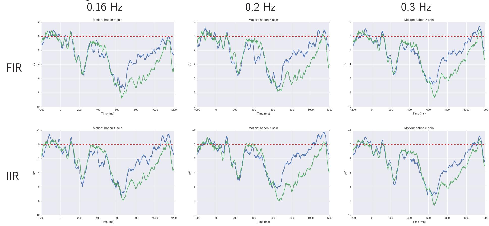
Using MNE in Python [10], we examined the effect of impulse-response type (**FIR vs. IIR**) and lower passband edge (0.16 vs. 0.2 vs. 0.3 Hz), while holding the upper passband edge constant at 30 Hz and using a 200ms pre-stimulus baseline correction. Zero-phase was achieved by forward-backward filtering.
